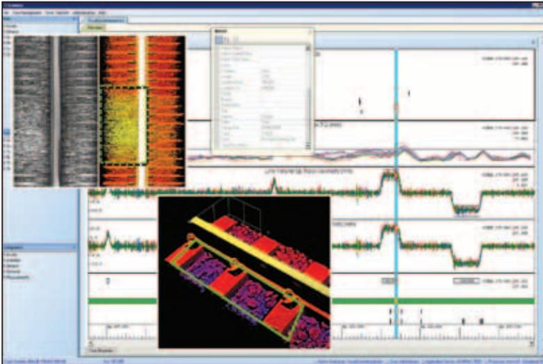
**Fig 1. Correlation of detected ballast and track geometry defects.**
