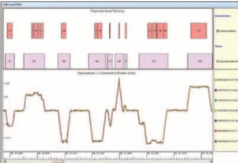
**Fig 2. Integrated visualisation of design and measured cant parameters.**
